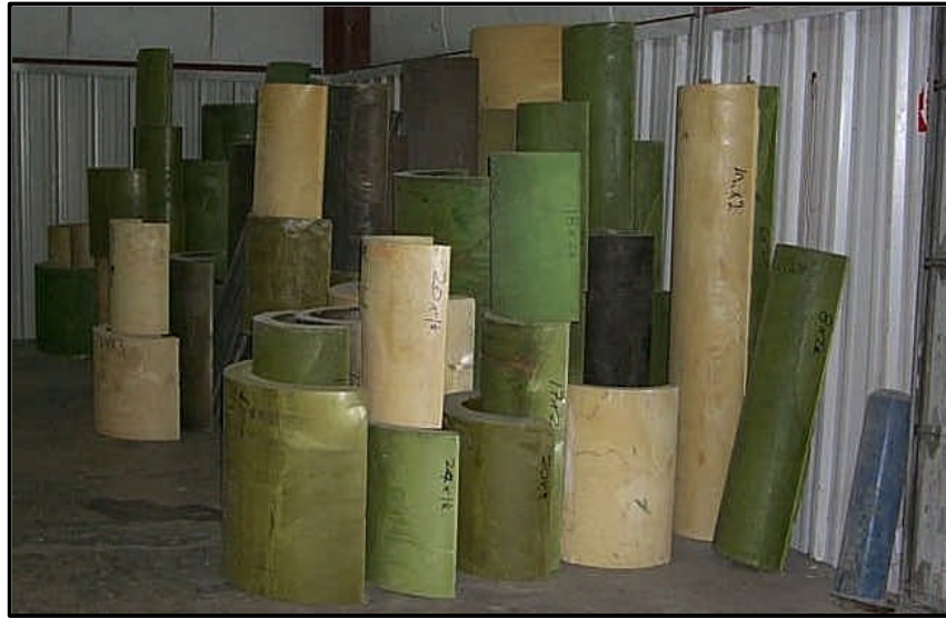
Polyurethane Forms cut into various lengths
