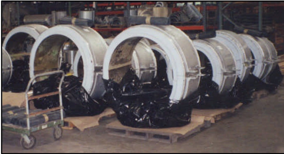
Large Diameter Coldshoe ready for shipment
