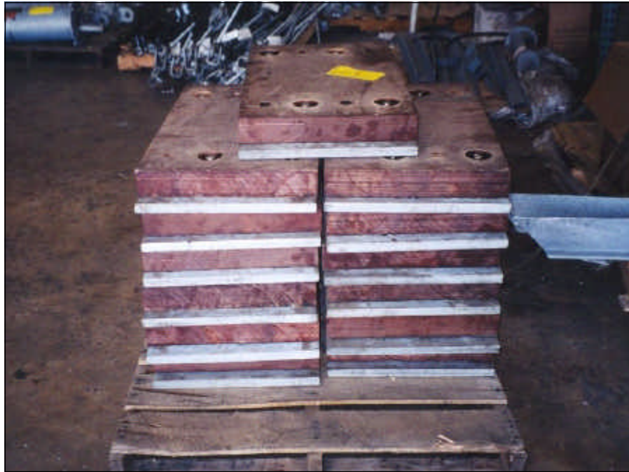
Phenolic Blocks awaiting further assembly
