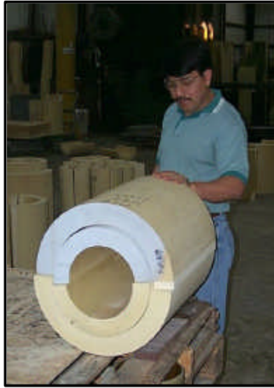
Manufactured Coldshoe being inspected for proper fit
