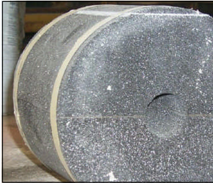
Foamglas ® formed to accommodate a 2" pipe
