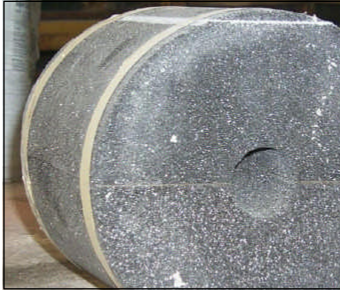
Foamglas formed to accommodate a 2" pipe
