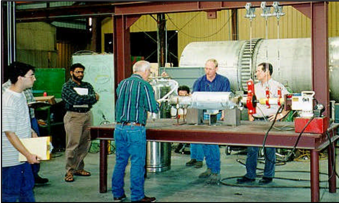
Testing of Load on a Pre-Insulated Support
