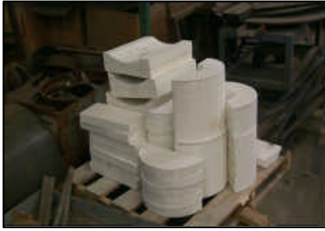
FireTemp® Shapes and Blanks used to Fabricate Hobbos
