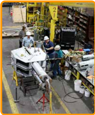
Damaged components repaired and both units rebuilt to original specifications
